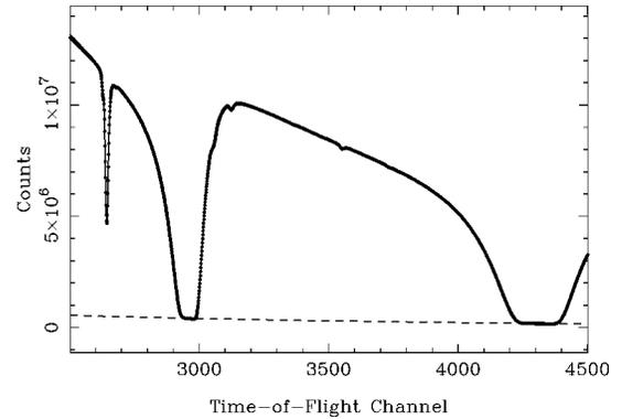
FIG. 1. The time-of-flight spectrum for  $^{133}\text{Cs}$  for the energy region from 22 eV to 79 eV. The channel width is 200 ns and the detector counts are summed for two helicity states over 45 runs.
