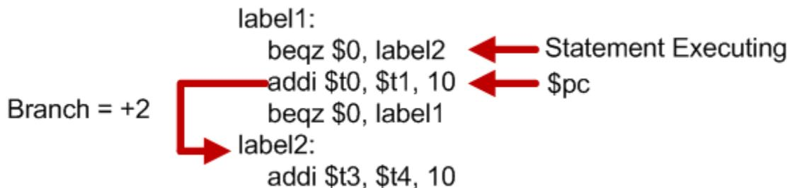
The second branch instruction branches backward to `label1`. In this case, the distance between the instruction and the label is -2 instructions, which is 2 words or 8 bytes, back from the current
