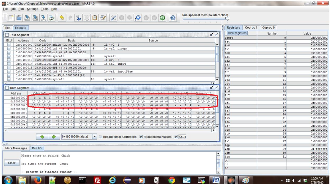
characters used) is the position of the first zero, or null. Thus strings are referred to as "null terminated". Many HLL, like C and C++<sup>7</sup>, use this definition of a string.
