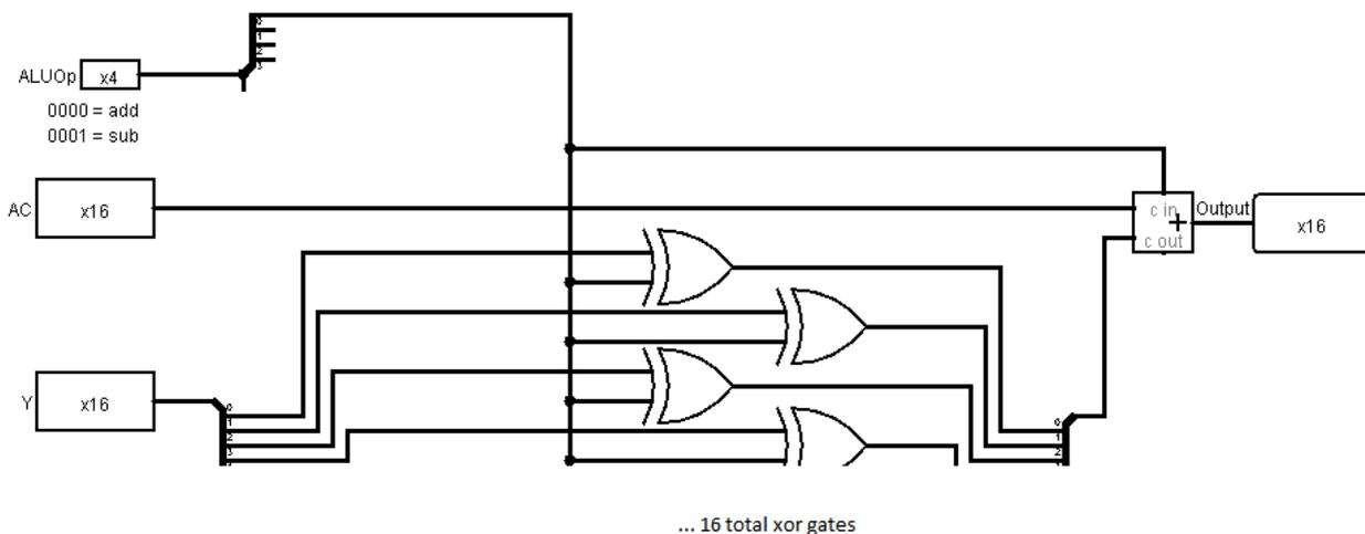
Figure 5-3: Adder/Subtractor
