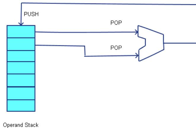
Figure 1-5: 0-address architecture
