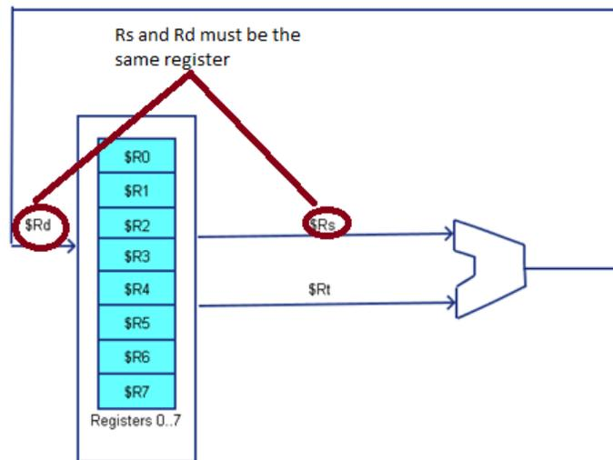
Figure 1-7: 2-address architecture
