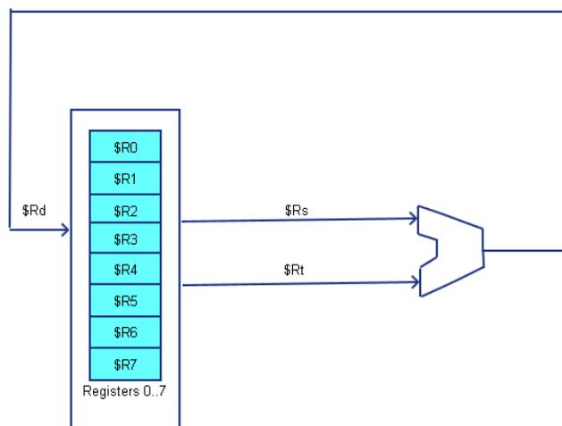
Figure 1-6: 3-address architecture
