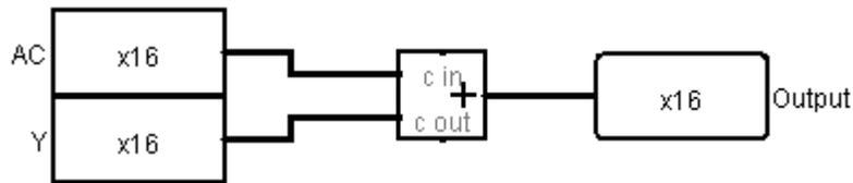
Figure 5-2: Simple Adder
