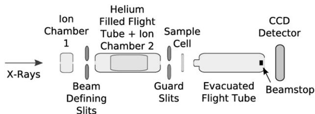
FIGURE 1 Schematic of the CHESS C-1 beamline, configured for ASAXS.
