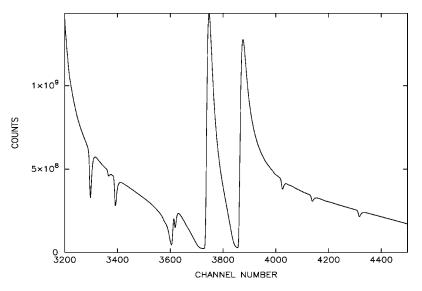
FIG. 1. Time-of-flight spectrum of thorium in the energy range 83–164 eV. The detector counts are the transient recorder readings with a channel width of 100 ns.
