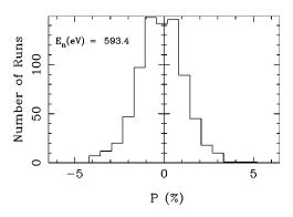
FIG. 5. Histogram of the *P* values for the 593.4-eV resonance in  $^{106}\text{Pd}$  for 784 30-min runs. The mean value from the distribution is given by  $P=-0.174\pm0.044,$  where the uncertainty is given by  $\sigma_{\text{sdev}}/\sqrt{784}.$
