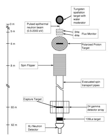
FIG. 1. Schematic of the TRIPLE beam line set up for a capture  $\gamma$ -ray measurement.
