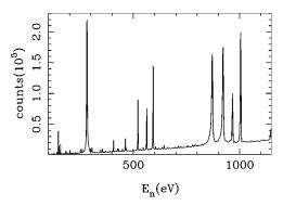
FIG. 2. A capture yield spectrum for  $^{106}\text{Pd}$  for neutron energies from 100 to 1150 eV.
