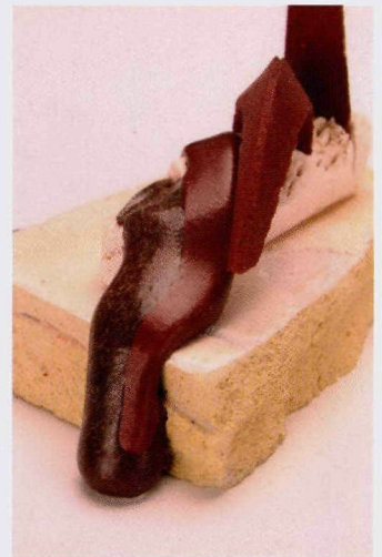
Stages of cone melt: Fluid glaze, stiff glaze (or engobe), and bending clay.
