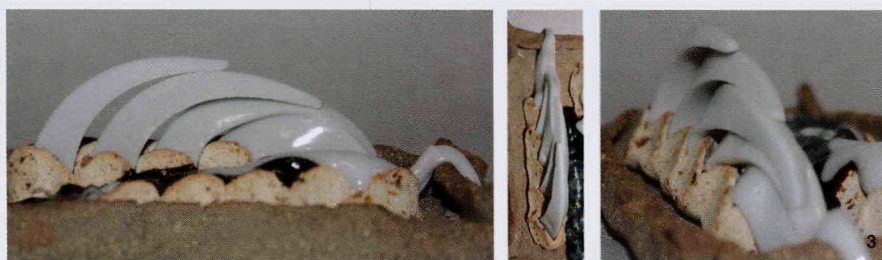
3 Cones will hit each other when aligned bending-face-to-spine, making it impossible to discern how far cone 11 has bent. The far left cone here is cone 11. Is it bent halfway? Or would cone 11 be down if cone 10 were not holding it up?
