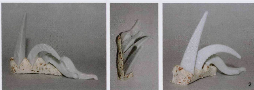
2 Cones can bend freely when aligned properly with spines and side faces in a continuous line, allowing easier and more accurate reading of the bend.
