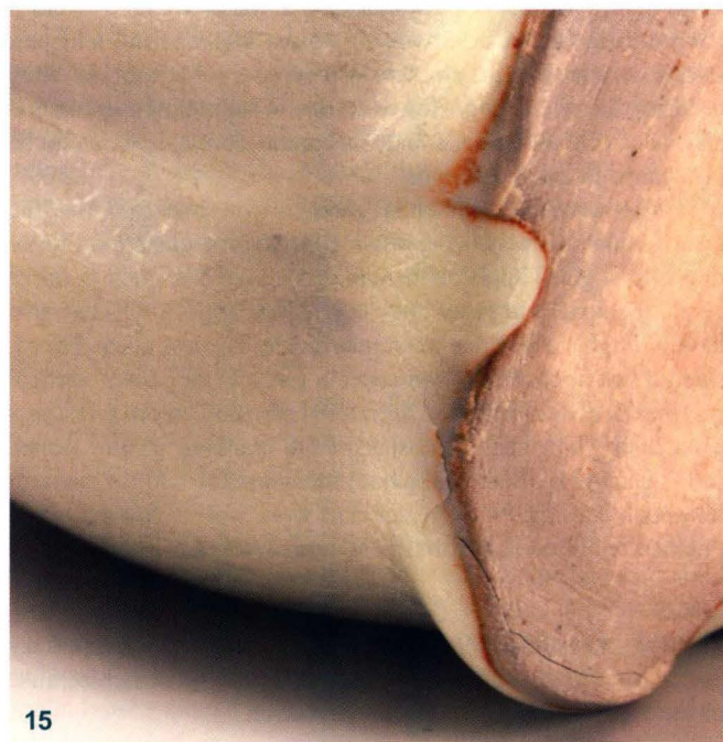
Material Doctors, Gebhart: 13 "SM-2C" puck grid. Two glaze dips, fired cold at c/10 half (c/10 down by unloading time); 2014, Photo by Meagan Lupolt, Research Assistant. 14 Glaze Sample, grid of mini pots: "T2" with Interface Cracking, 2014, detail; Photo by Meagan Lupolt, Research Assistant. 15 Glaze Sample, small pot: "T2" with Interface Cracking, 2014, detail; Photo by Tina Gebhart. 16 Tina Gebhart: Pumpkinned Ewer 8x7x5" Porcelain, 2014. 17 Tina Gebhart: Hip Hugger Mug 6x5x4" Porcelain, 2014. Photos 16 & 17: Tina Gebhart
