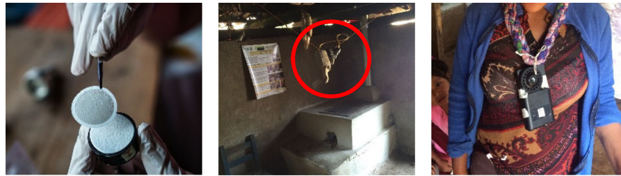
A PM 2.5 Air sampling filter after 24-hours of household air pollution monitoring. B Kitchen exposure equipment hanging near the Justa cookstove: pump, triplex cyclone, temperature logger; Justa training poster on wall. C Personal exposure equipment (UPAS) with accelerometer taped to the back, worn by a participant.
