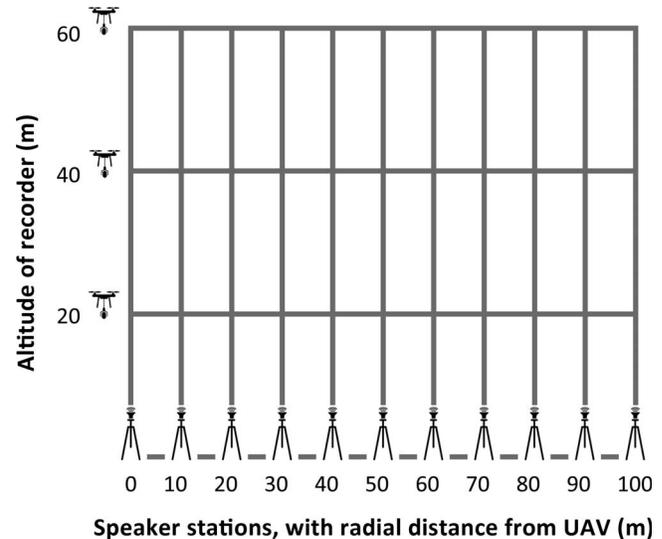
**FIGURE 1.** Experimental setup for protocol development. We attached an audio recorder to an unmanned aerial vehicle (UAV), which was flown at 3 altitudes while songs were played at random from 11 speaker stations located at regular intervals within 100 m radial distance from where the UAV hovered.
