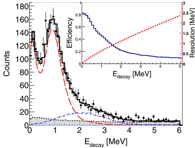
FIG. 1. Two-body decay energy for  $^{22}\text{N} + 1n$ . The best fit includes two-channel Breit-Wigners resulting from two states at 1.1 MeV (dashed-red line) and 2.4 MeV (dot-dashed-blue line). Background contributions are in shaded gray. The efficiency and resolution are shown in the inset as the blue histogram (left scale) and red-dashed line (right scale), respectively.
