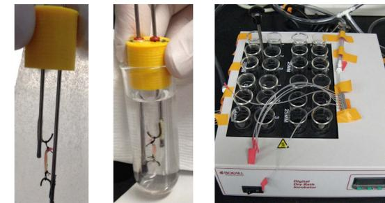
Figure 5. Mounted skeletal muscle (left), *in vitro* incubation apparatus (middle), and heat block (right).
