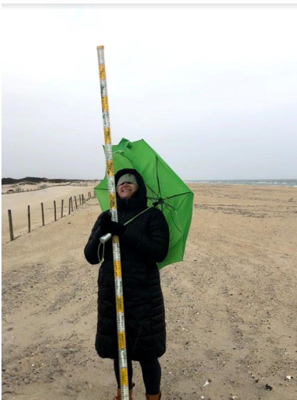
Figure 2c. An example of the meter stick/pole that was used to conduct the beach profiles.
