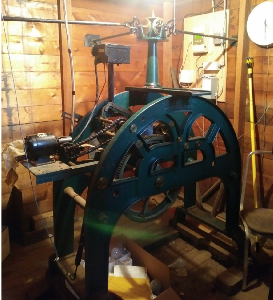
The original gears of the bell and clocks. This is still used in part for the clock and bell mechanisms. Picture taken by author, September 21, 2018.
