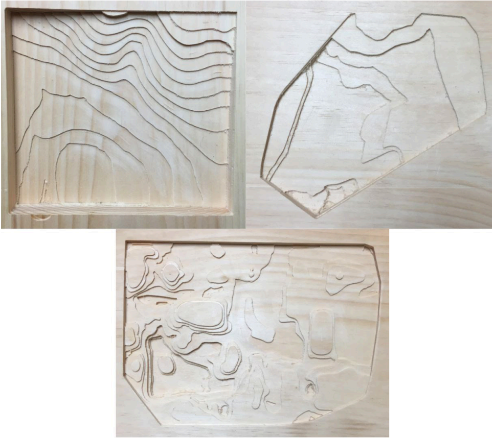
Figure 11. (Top left to right) Wooden models of Area 3 of Boyer Orchard, Quarry Pond, and Stine Lake/West Quad created using computer numerical controls of the Carvey Inventables 3D Carver.
