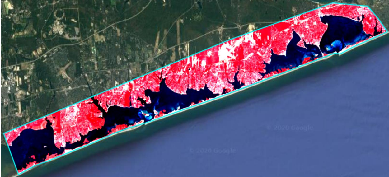
Figure 3. This is a color infrared (CIR) composite image from 28 Landsat images displaying the study area before the creation of the new inlet (images from July 2008 to August 2012). Prior to the creation of the inlet, the Bellport Bay (left of study area) lacks the flashes of white/blue seen adjacent to the inlets of the Moriches(middle) and Shinnecock Bays (right).
